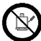
Never open the emulator box for any reason whatsoever, especially with the engine running or the panel switched on.
