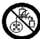
Install far from the ignition coil and pass the wiring far from the high voltage cables.
