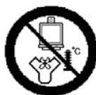
Install far from any sources of excessive heat (eg. exhaust manifold).
